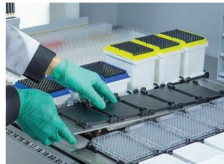
Exchange deck segments for flexible assay set-up, device integration and reconfiguration
